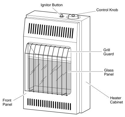
Figure 1 - Vent-Free Natural Gas Heater
